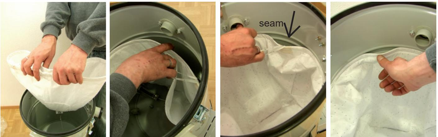
Before insertion of the new filter, the hook has to be fastened again. To insert the filter, the filter must be formed to a semi-circle and be placed gently into the seam.
