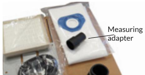
Insert the measuring adapter into the valve. Be sure to check that all other valves are closed and the suction hose is not attached.
