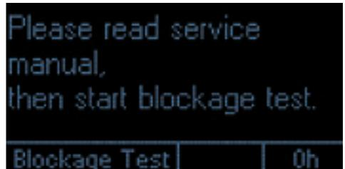
Press the power button on your central vacuum cleaner. The blockage test starts. An index value is determined for this valve.
